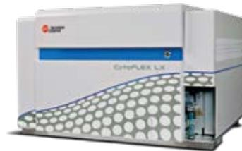
... optimally combines excitation and emission, thereby achieving maximum sensitivity. Detection of extracellular vesicles; Measurement of bacteria, bacteriophages, yeasts, cells or similar can be easily realized. With up to 6 lasers and up to 21 fluorescence avalanche photo diodes (plus 2 scatters) this system leaves nothing to be desired.
